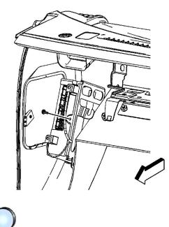
4. Remove the screw retaining the VCIM to the bracket.
